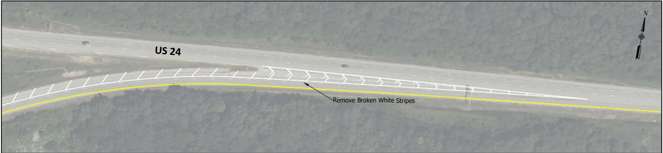
Proposed striped gore area on existing two-lane ramp to reduce to one 16' ramp lane
