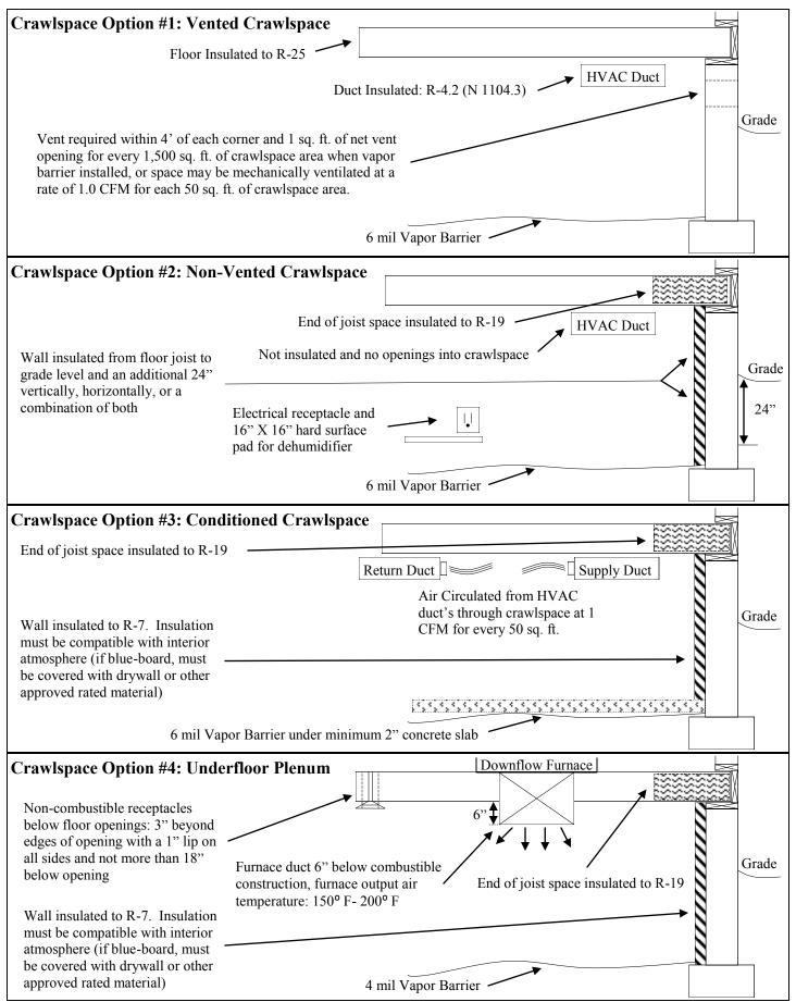
\*All options require that crawlspace floor (gravel or concrete) be sloped to the required sump pit
