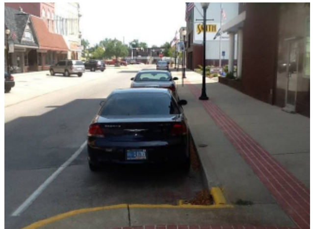
Photo illustrates on-street parallel parking on Jefferson St. Space with barrier-free sign not near curb ramp.
