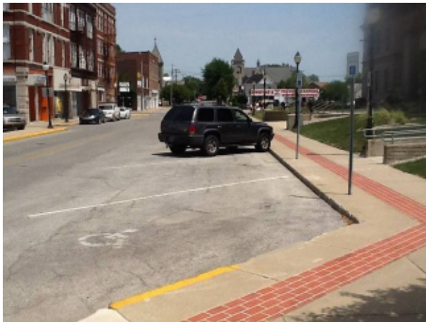
Photo illustrates on-street angled parking on Franklin St. Access aisles not provided between adjacent spaces.
